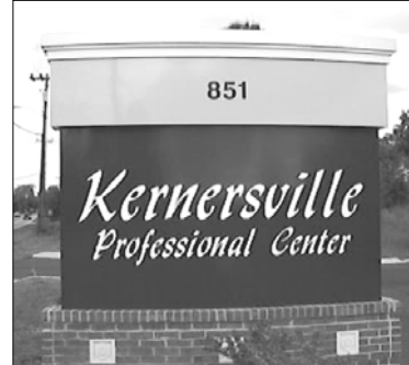
Example of a knockout backlit sign
